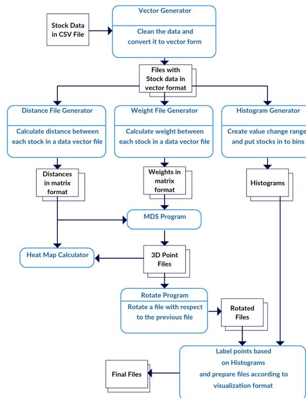
Fig 1. Data analysis pipeline
