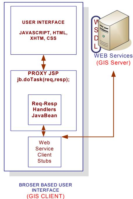
Figure 1: Invoking Web Services from the AJAX applications.
