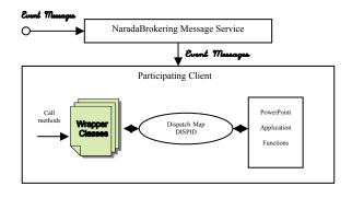
Fig. 2 the event messages invoke methods of wrapper class; the methods then are mapped to functions of PowerPoint application through Dispatch Map/DISPID; the functions are executed and result/status code are returned.
