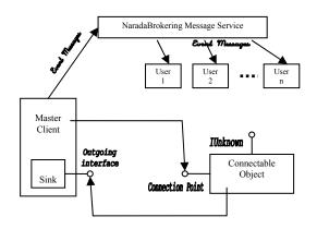
Fig. 1 Connectable Object calls outgoing interface implemented by the sink. Master client handles events fired from the connectable object through the sink, and sends them to the message broker which then distributes to participating users
