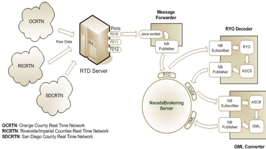
**Figure 3 GPS real-time data filtering is accomplished using NaradaBrokering filter chains.**
