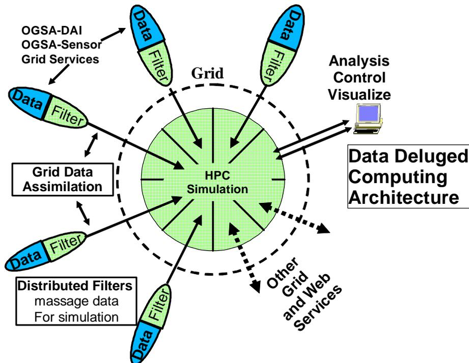
**Figure 1:** The figure illustrates the hub and spoke architecture for assimilating data using extreme scale computing. Distributed data sources use local clusters for adaptively filtering data, which is then transported using high-performance transport services to one or more centralized high performance computers.
