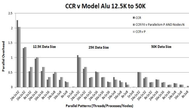
**Fig. 8.** Parallel Overhead  $f$  as a function of pattern  $t \times m \times n$  for three samples of respectively 12,500 25,000 and 50,000 AluY sequences in the case  $m=1$  of threading internal to node. We show for each pattern, the CCR measurement followed by the two factor and single factor model.
