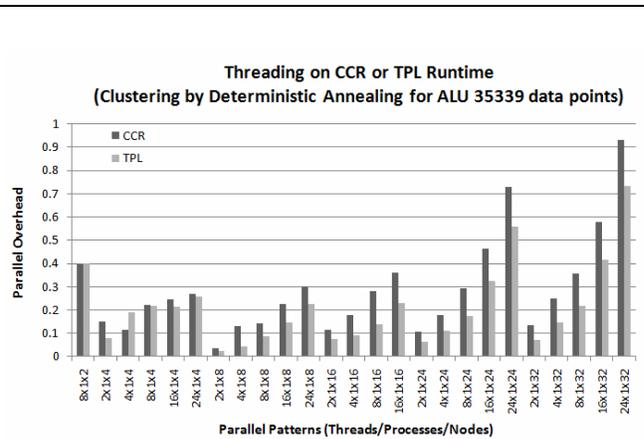
**Fig. 5. Parallel Overhead for 35399 AluY sequence clustering for cases of pure threading in the node**
