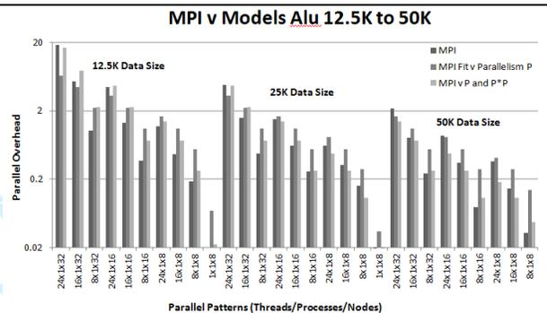
**Fig. 11.** Parallel Overhead  $f$  as a function of pattern  $t \times m \times n$  for three samples of respectively 12,500 25,000 and 50,000 AluY sequences in the case  $t=1$  of MPI internal to node. We show for each pattern, the CCR measurement followed by the single factor and two factor model.
