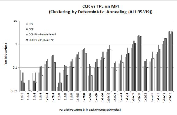
**Fig. 10.** Parallel Overhead for 35399 AluY sequence clustering for cases of pure MPI internal to the node. For each pattern, we show in order the measured TPL, the measured CCR, the single factor model CCR prediction and finally the two factor model CCR prediction.
