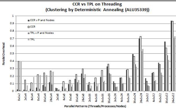
**Fig. 7.** The data of Fig. 5 compared with a simple model described in text for MPI and threading. For each pattern, we show in order the model CCR prediction, the measured CCR, the model TPL prediction and finally the measured TPL
