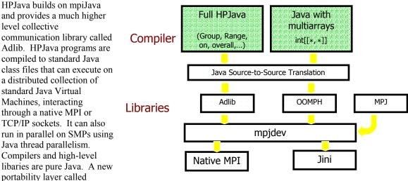
mpjdev encapsulates any unavoidable platform dependence.
