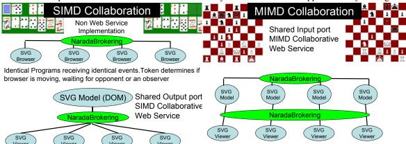
either the input or output ports of the web service. We have applied this to the Java SVG (Scalable Vector Graphics) browser and to PowerPoint; the former is a complete Web service implementation using userinteraction events; the latter uses higher-level semantic events like "slide change". We believe a complete Web Service architecture desktop can be built this way and that it
