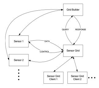
Figure 1. A Collaborative Sensor Grid Architecture
