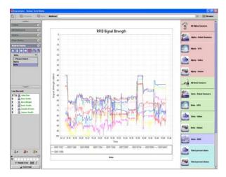
Figure 12. A UDOP shows and shares RFID signal strength of ten active RFID tags
