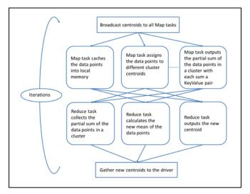
Figure 2. K-means Clustering execution flow in Twister
