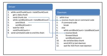
Figure 8. The algorithm steps per chain
