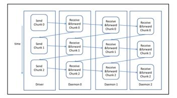
Figure 9. The execution flow per chain
