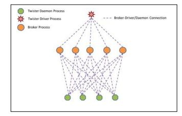
Figure 5. Unconnected broker array with 5 brokers and 4 daemon nodes
