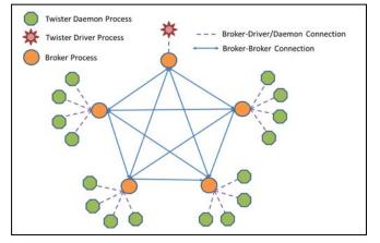
Figure 4. Full mesh broker network topology with 5 brokers and 16 daemon nodes
