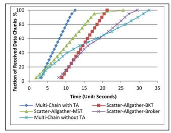
Figure 12. CDF of the received data chunks on 125 nodes under different broadcast methods (TA: Topology-Awareness)
