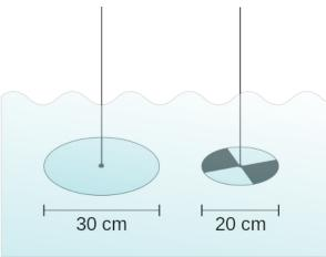
Figure: Secchi disk types. A marine style on the left and the freshwater version on the right wikipedia.
