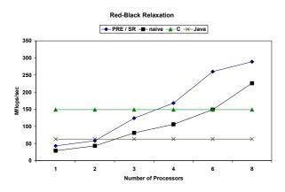
Figure 5. Laplace Equation with red-black relaxation with size of 512 x 512 on Sun Solaris 9 with 8 UltraSPARC III processors.
