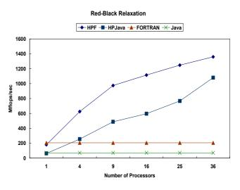
Figure 6. Laplace Equation with red-black relaxation with size of 512 x 512 on IBM SP3.
