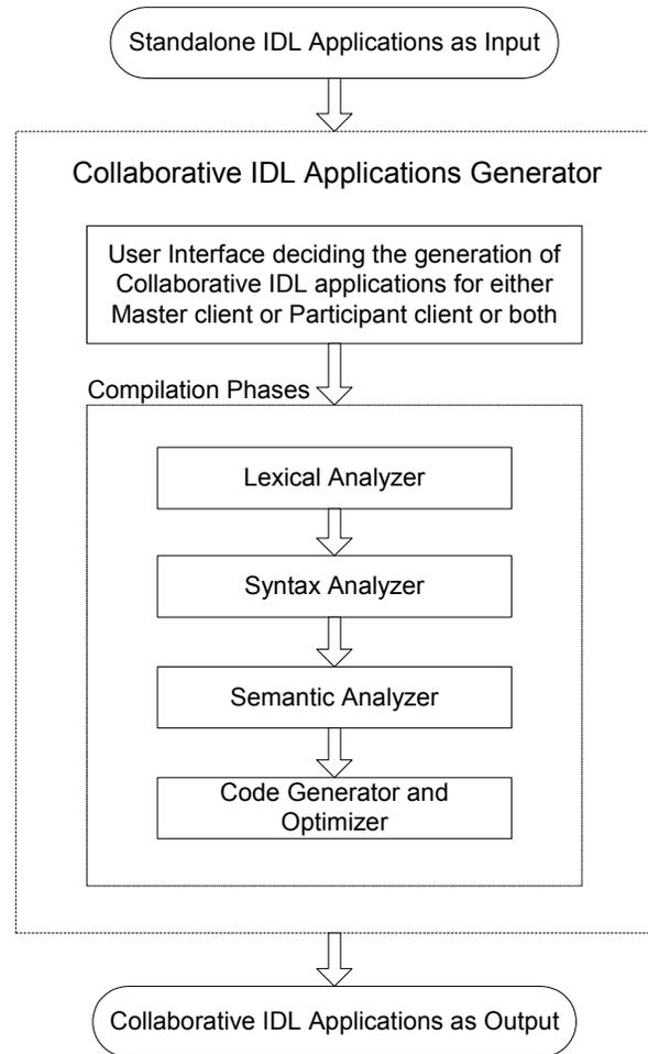
**Figure 2. Dynamic structure for generating collaborative IDL applications**
