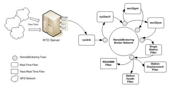
Fig. 2. The filter chain architecture used to process streaming GPS data. Several format conversion filters process the data before it is sent to the RDAHMM software that performs the HMM-based time series analysis.
