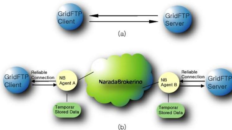
Figure 1 (a) Traditional GridFTP (b) GridFTP with NaradaBrokering
