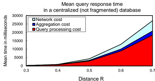
**Fig. 4.** Mean query response time between a web service client and a centralized database host server including the corresponding execution time of the middleware and agents, varying the distance  $R$ .
