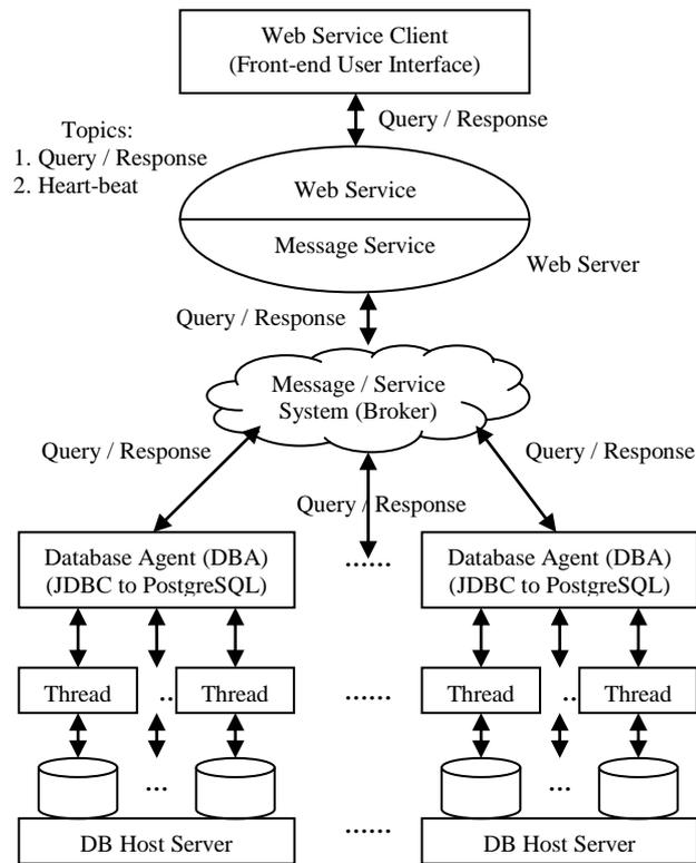
**Fig. 1.** Scalable, distributed database system architecture - three tiers: web service client, web service and broker, and agents and a collection of databases.
