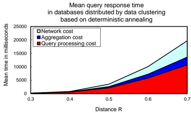
**Fig. 7.** Mean query response time between a web service client and databases distributed by data clustering including the corresponding execution times of the middleware and agents, varying the distance  $R$ .
