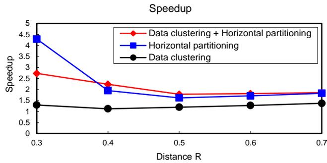
**Fig. 5.** The value of speedup is the mean query response time in a centralized database system over the mean query response time in a distributed database system.
