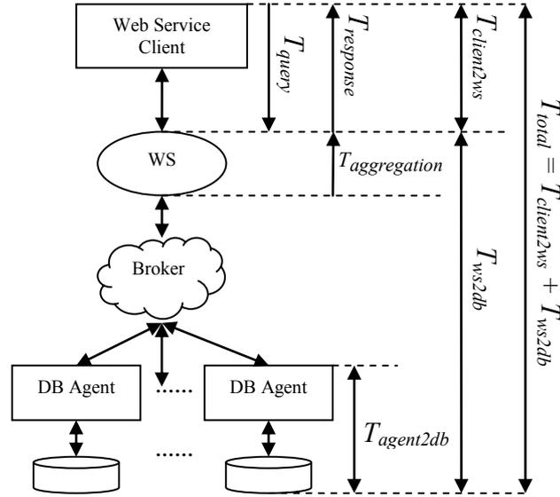
**Fig. 3.** Total latency ( $T_{total}$ ) = Transit cost ( $T_{client2ws}$ ) + Web service cost ( $T_{ws2db}$ )
