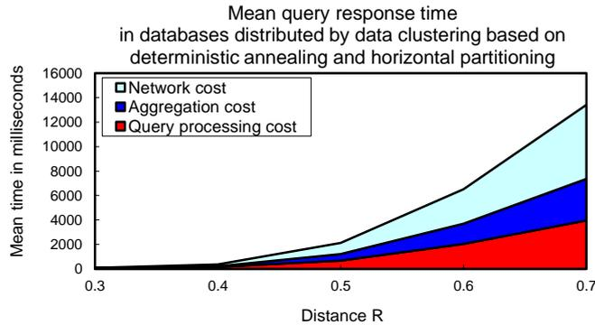
**Fig. 9.** Mean query response time between a web service client and databases distributed by data clustering and horizontal partitioning including the corresponding execution times of the middleware and agents, varying the distance R.
