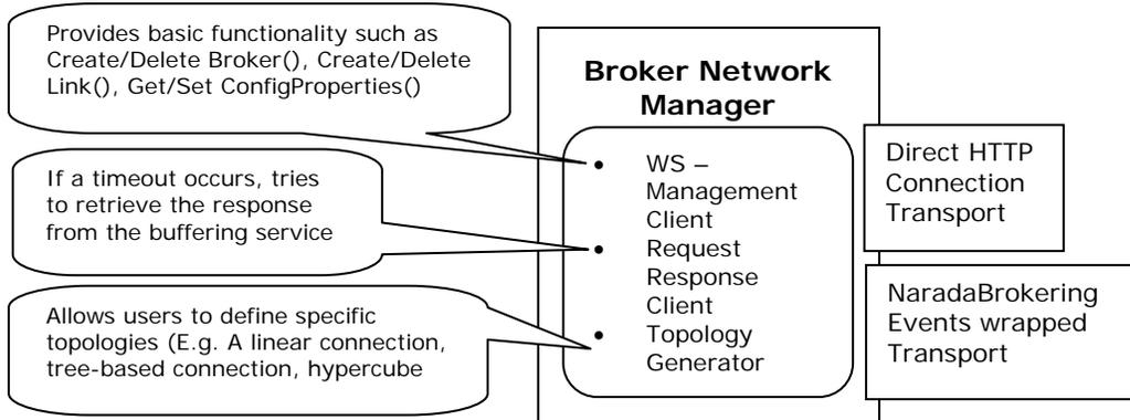
**Figure 4:** Broker Network Manager (aids in deployment of Broker network)
