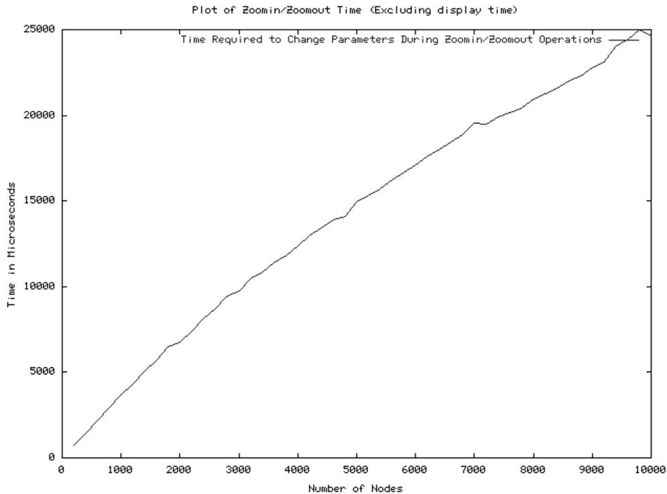
Fig.11. Time Required for Zooming Operations against Number of Nodes in System
