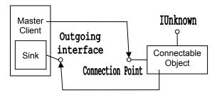
Figure 2. Connectable object calls outgoing interface implemented by the sink. Master client handles events fired from the connectable object through the sink.
