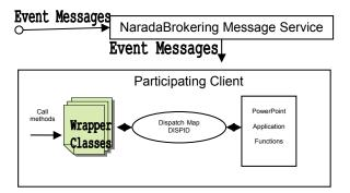
Figure 3. The event messages invoke methods of wrapper classes; the methods are mapped to functions of PowerPoint application through Dispatch Map/DISPID, which are then executed and results/status codes are returned back.
