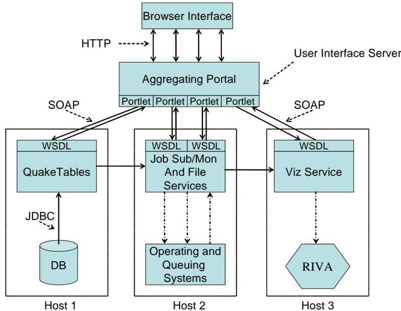
Figure 1 SERVO Grid is built using component-based portals and Web Services. This shows a job submission and management service linked to data service (Fault database Quaketables) and a visualization service. The user interfaces to this set of Grid Services is provided by an aggregation portal whose portlet architecture supports a component model of user interfaces illustrated in fig. 2.
