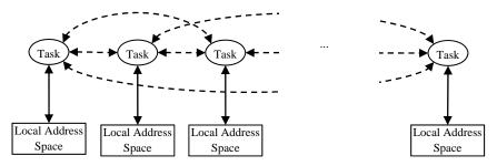
Figure 6. Programmer's view of distributed memory model
