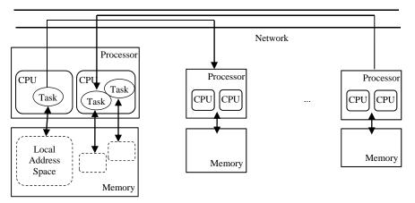
Figure 7. Architecture of distributed memory model implementation
