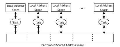
Figure 10. Programmer's view of a PGAS model
