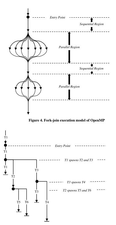
Figure 5. Execution model of a Pthread program
