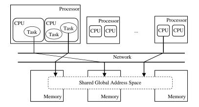
Figure 3. Architecture of shared memory model implementation
