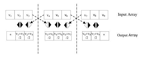
Figure 12: Local view of a 3-point stencil computation
