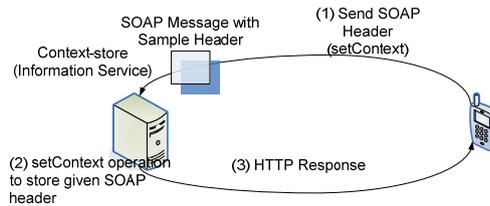
**Fig. 8.** Set up for measuring Context-store accessing overhead
