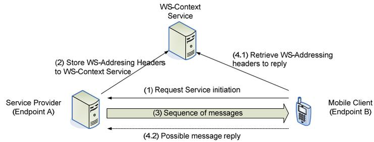
Fig. 10. Scenario for WS-Addressing example
