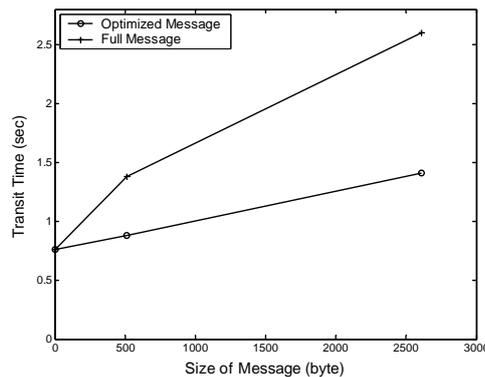
Fig. 12. Round trip time of optimized message exchange through the HHFR high performance channel compared with full message exchange
