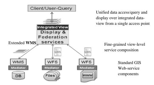
Figure 2: Data life-cycle and integrated data-view creation.
