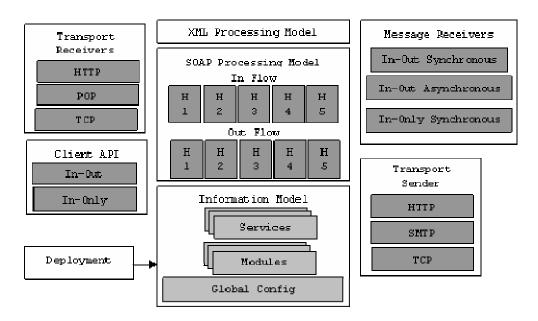
Figure1: Axis2 Architecture
