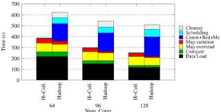
Figure 5. MDS Hadoop using only the BC Calculation MapReduce job per iteration to highlight the overhead. 20 iterations, 51,200 data points.
