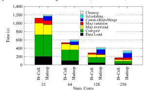
Figure 10. Hadoop MapReduce K-means Clustering & H-Collectives Map-AllReduce Strong scaling. 500 Centroids, 20 Dimensions, 10 iterations.
