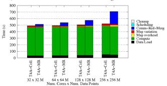
Figure 11. Twister4Azure K-means weak scaling with Map-AllReduce. 500 Centroids, 20 Dimensions. 10 iterations. 32 to 256 Million data points.
