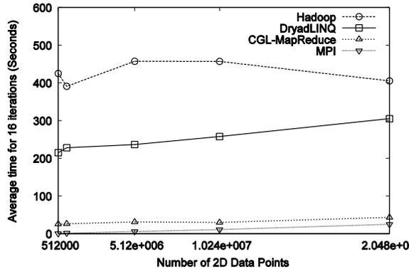
Figure 7. Overhead induced by different parallel programming runtimes for the Kmeans Clustering application – overhead against the number of 2D data points clustered (Note: Both axes are in log scale)
