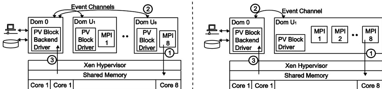
Figure 18. Communication between dom0 and domU when 1-VM per node is deployed (left). Communication between dom0 and domUs when 8-VMs per node were deployed (right).
