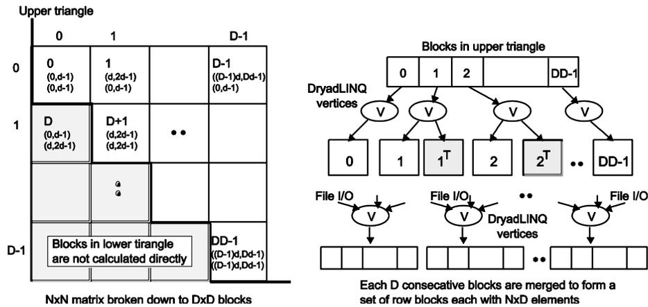
Figure 3. Task decomposition (left) and the DryadLINQ vertex hierarchy (right) of the DryadLINQ implementation of SW-G pairwise distance calculation application.
