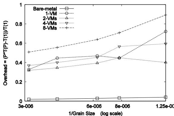
Figure 14. Total overhead of the Kmeans clustering – overhead against the 1/ grain size, grain size = number of 2D data points per parallel task (Number of MPI Processes = 128 )
