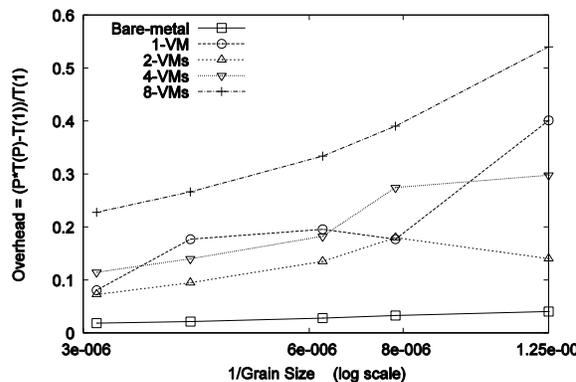
Figure 15. Parallel overhead of the Kmeans clustering – parallel overhead against 1/grain size (Number of MPI Processes = 128 )
