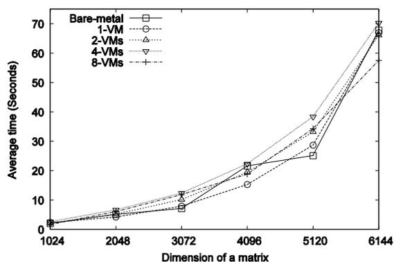
Figure 10. Performance of the matrix multiplication application – average time (in seconds) against the size of a matrix (Number of MPI processes = 64).
