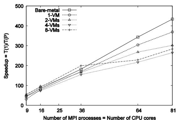
Figure 11. Speed-up of the matrix multiplication application – Speedup against the number of MPI processes = number of CPU cores used (Fixed matrix size = 5184x5184).
