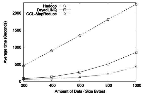
Figure 5. Performance of the CAP3 application – average time (in seconds) against the number of gene reads processed.
