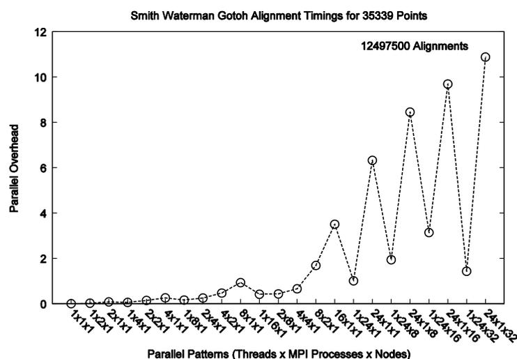
Figure 9. Performance of ALU Gene Alignments for different parallel patterns
