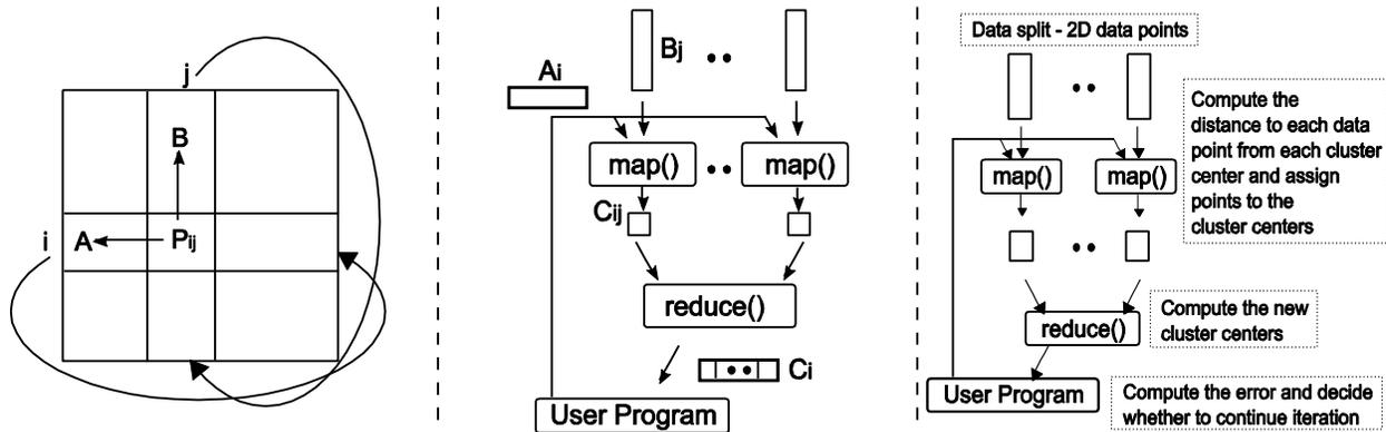
Figure 2. (Left) The communication topology of Cannon's Algorithm implemented using MPI, (middle) Communication topology of matrix multiplication application based on MapReduce, and (right) Communication topology of Kmeans Clustering implemented as a MapReduce application.
