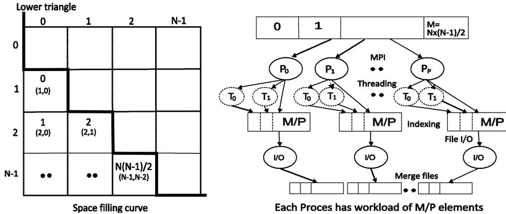
Figure 4. Task decomposition (left) and the MPI (right) implementation of SW-G pairwise distance calculation application.
