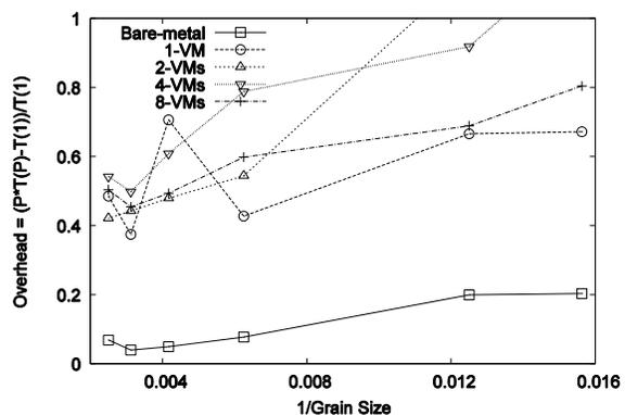
Figure 17. Total overhead of the Concurrent Wave Solver – overhead against 1/grain size, grain size = number of points assigned per parallel task (Number of MPI Processes = 128 )
