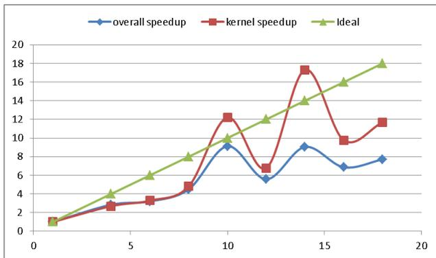
Figure 5: Speedup of MPI/OpenMP implementation of C-means on multiple GPUs.
