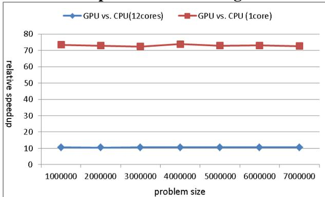
Figure 2: relative speedup of GPU implementation as compared to CPU implementation with 12 cores and 1 core respectively.
