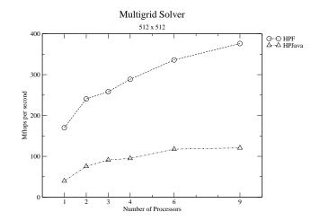
**Fig. 9.** Multigrid solver with size of  $512^2$ .
