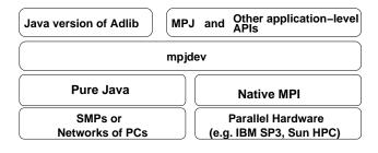
Fig. 1. An HPJava communication stack
