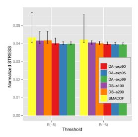
Fig. 5. The normalized STRESS comparison of **yeast** data mapping results in 2D space. Bar graph illustrates the average of 50 runs with random initialization and the corresponding error bar represents the minimum and maximum of the normalized STRESS value of SMACOF, DS-s100 and s200, and DA-exp90,DA-exp95, and DA-exp99. The x-axis is the threshold value for the stopping condition of iterations  $(10^{-5} \text{ and } 10^{-6})$ .
