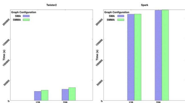
Fig. 6. Execution time for Source-Map-AllReduce (SMA) and Source-Map-Map-AllReduce(SMMA) graph configurations. With 200K data points and 100 iterations
