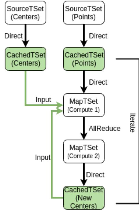
Fig. 3: K-Means TSet API dataflow graph
