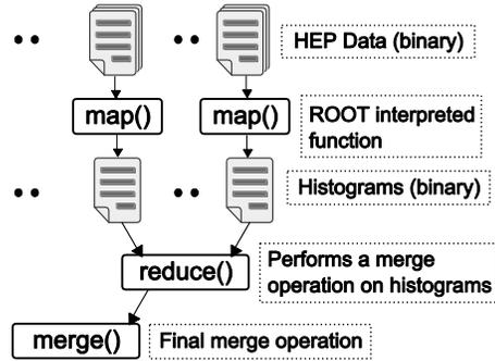
Figure 4. MapReduce for the HEP data analysis
