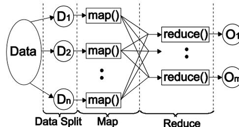
Figure 1. The MapReduce programming model
