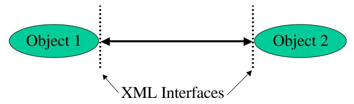
The basic approach is the same whatever the object model: COM, CORBA, Jini/RMI, SOAP(.net), or even DMSO's HLA. In each case, systems are built in multi-tier fashion so the front end rendering and back end functionality are disassociated In the picture below, we show an example of a software object being defined in XML.
