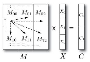
Fig. 3. Parallel matrix multiplication of  $N \times N$  matrix and  $N \times L$  matrix based on the decomposition of Fig. 2
