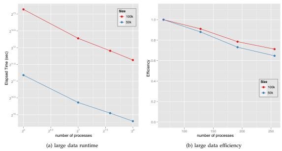
Fig. 8. Performance of parallel SMACOF for 50K and 100K PubChem data in Cluster-II w.r.t. the number of processes, i.e. 64, 128, 192, and 256 processes (cores). (a) shows runtime and efficiency is shown at (b). We choose balanced decomposition as much as possible, i.e.  $8 \times 8$  for 64 processes. Note that both x and y axes are log-scaled for (a).
