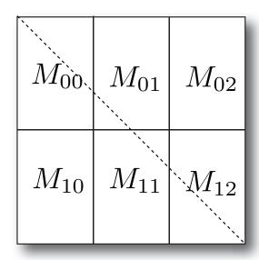
Fig. 2. An example of an  $N\times N$  matrix decomposition of parallel SMACOF with 6 processes and  $2\times 3$  block decomposition. Dashed line represents where diagonal elements are.
