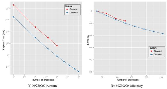
Fig. 11. Performance of parallel SMACOF for MC 30000 data in Cluster-I and Cluster-II w.r.t. the number of processes, i.e. 32, 64, 96, and 128 processes for Cluster-I and Cluster-II, and extended to 160, 192, 224, and 256 processes for Cluster-II. (a) shows runtime and efficiency is shown at (b). We choose balanced decomposition as much as possible, i.e.  $8 \times 8$  for 64 processes. Note that both x and y axes are log-scaled for (a).
