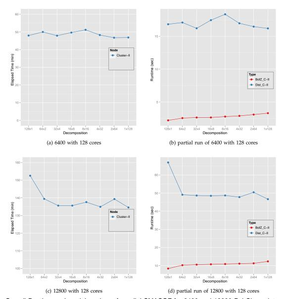
Fig. 7. Overall Runtime and partial runtime of parallel SMACOF for 6400 and 12800 PubChem data with 128 cores in Cluster-II w.r.t. data decomposition of  $N \times N$  matrices.
