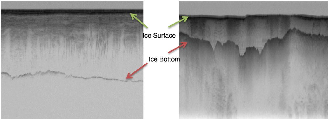
Fig. 1. Ice surface and bottom depicted in radar echograms gathered by the Multichannel Coherent Radar Depth.
