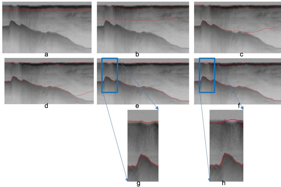
Fig. 3. Contour evolution throughout processing. a) Initial curve, (b)-(e) contour adaptation to ice surface and bottom layers after 200, 400, 600, and 800 iterations correspondingly, (f) manually picked interfaces, (g)-(h) the magnified section of (e) and (f)
