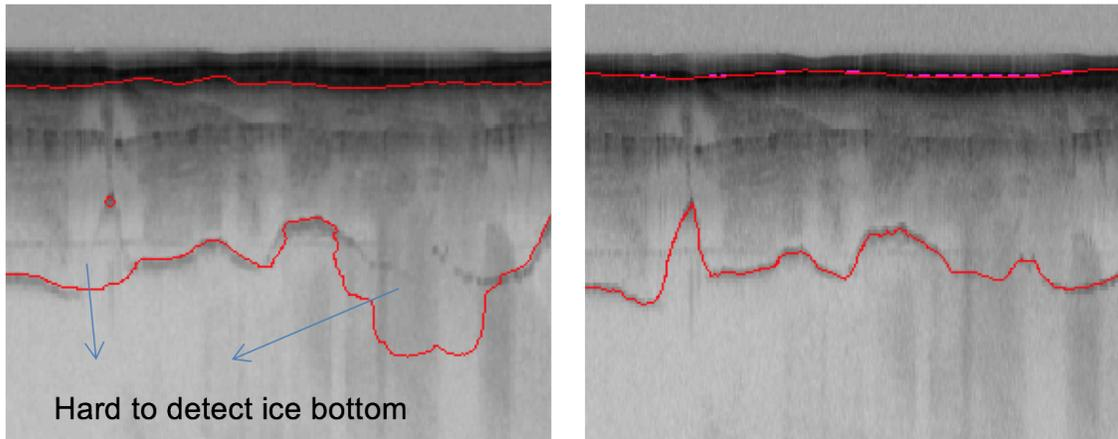
Fig. 6. Our approach is not able to detect the invisible parts of ice bottom, left: the ice surface and bottom detected by our approach, right: manually picked interfaces
