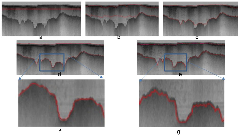
Fig. 4. Contour evolution throughout processing. a) Initial curve, (b)-(d) contour adaptation to ice surface and bottom after 200, 400, and 800 iterations correspondingly, (e) manually picked interfaces, (f)-(g) the magnified section of (d) and (e)
