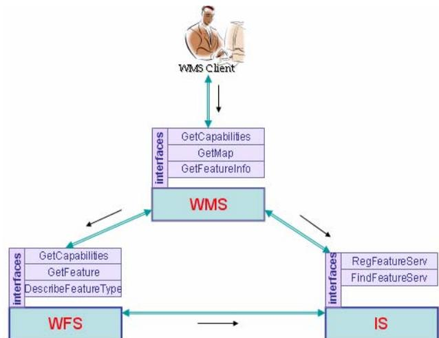
Figure 4 : Basic GIS Components Involved in Visualization System.
