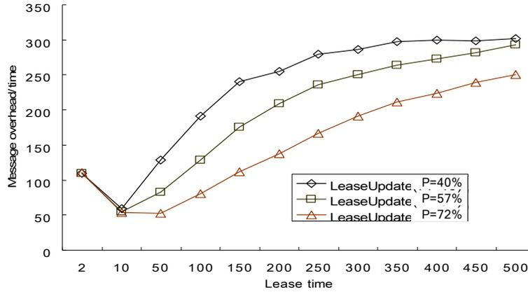
Fig. 21 Message Overhead for the variable period ratio ( $P = P_{bef\_wrt}$ )
