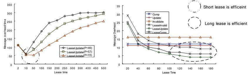
Fig. 29 Lease adjustment by data access pattern(  $P_r = P_{bef\_wrt}$  )
