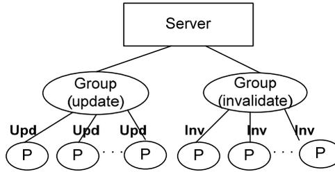
Fig.25 2-tier Notification structure by heterogeneous group
