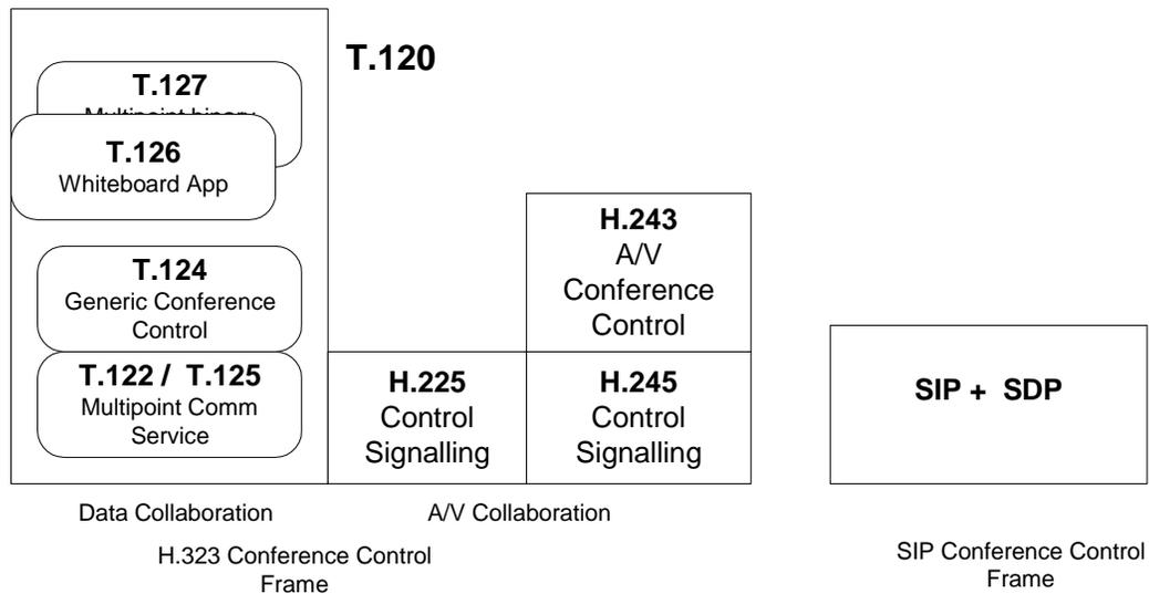
Figure 1 H.323, T.120 and SIP protocol stack
