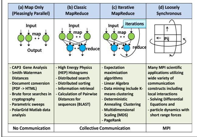
**Figure 3: Classification of Applications and Communication Patterns**
