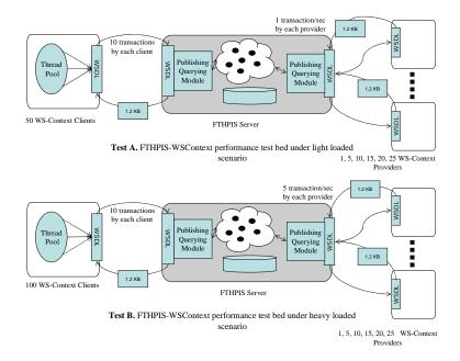
**Fig.17.** Experiments with varying number of concurrent clients and providers at various loads.
