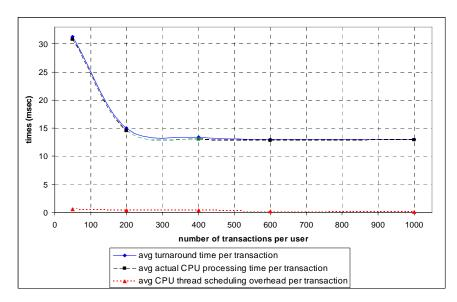
**Fig.19.** Measuring CPU Scheduling Latency spent in internal sub-activities of WS-Context inquiry function for 1 querying client under varying loads
