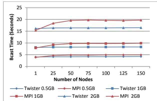
Figure 1. Chain Method/Open MPI MPI\_Bcast
