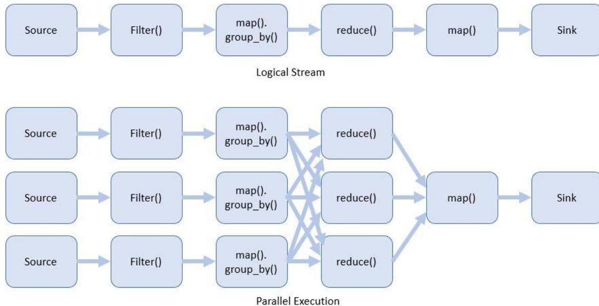
Figure 5. Flink logical task view and parallel execution view.
