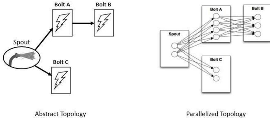
Figure 3. Storm/Heron topology. On the left is the abstract topology as defined by the program and on the right is the unrolled parallel topology for runtime.
