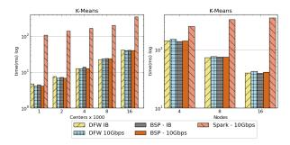
Fig. 10. Left: K-means job execution time on 16 nodes with varying centers, 2 million points with 320-way parallelism. Right: K-Means wth 4,8 and 16 nodes where each node having 20 tasks. 2 million points with 16000 centers used.
