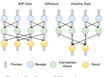
Fig. 1. Dataflow vs. BSP graph structure
