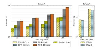
Fig. 11. Left: Terasort time on a 16 node cluster with 384 parallelism. BSP and DFW shows the communication time. Right: Terasort on 32 nodes with .5 TB and 1TB datasets. Parallelism of 320.
