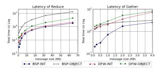
Fig. 9. Latency for OpenMPI and Twister:Net for Reduce and Gather operations in 32 nodes with 256-way parallelism. The time is for 1 million messages in each parallel unit, with the given message size
