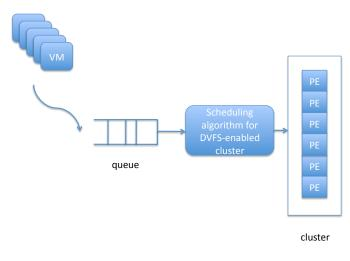
Fig. 3. Working scenario of a DVFS-enabled cluster scheduling
