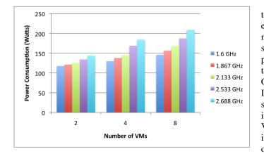
Fig. 5. Power consumption variations for a Intel Nehalem Quad-core processor
