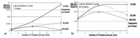
**Fig. 5.** Ratio of Standard Deviation to mean of thread execution time using Redhat on Intel8c (a,b) Linux and C with locks for synchronization on Clustering Kernel for three dataset sizes with 10,000 50,000 or 500,000 points per thread (core). Fedora shows larger effects than Redhat.
