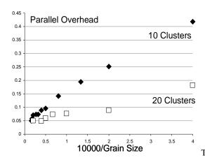
**Fig. 1.** Parallel Overhead for GIS 2D Clustering on Intel8b using C# with 8 threads (cores) and CCR Synchronization. We use two values (10, 20) for the number of clusters and plot against the reciprocal of the number of data points.
