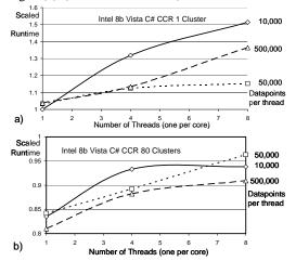
**Fig. 3.** Scaled Run time on Intel8b using Vista and C# with CCR for synchronization on Clustering Kernel for three dataset sizes with 10,000 50,000 or 500,000 points per thread(core). Each measurement involved averaging over at least 1000 computations separated by synchronization whose small cost is not included in results.
