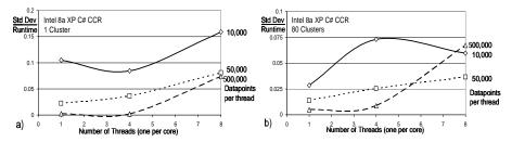
**Fig. 4.** Ratio of Standard Deviation to mean of thread execution time averaged over 1000 instances using XP on Intel 8a and C# with CCR for synchronization on Clustering Kernel for three dataset sizes with 10,000 50,000 or 500,000 points per thread (core).
