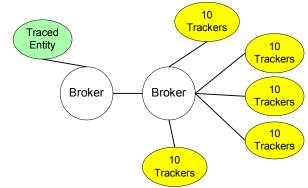
Figure 3: Topology for measuring effect of increasing number of trackers
