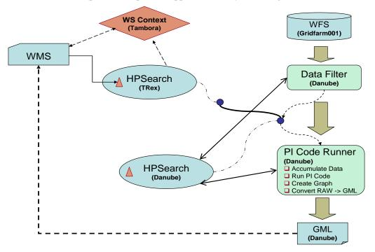
Figure 2 GIS Grid and Execution Grid services may be integrated into meta-applications using workflow orchestration tools such as HPSearch. This represents a "two-level" programming model: applications are
