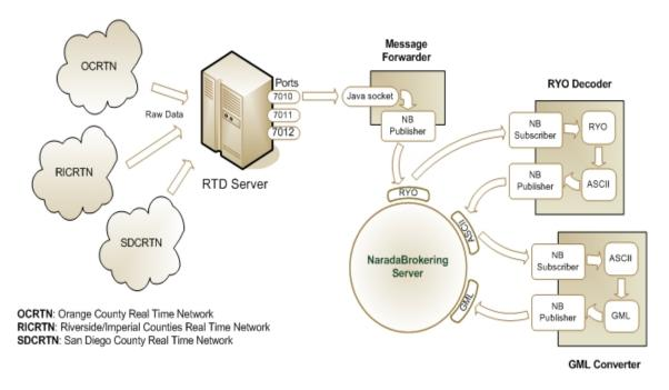
Figure 3 GPS real-time data filtering is accomplished using NaradaBrokering filter chains.
