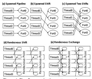
Figure 4. Five Communication patterns using CCR to test spawned dynamic threading (a,b,c) and MPI style Rendezvous's (d,e)
