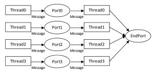
Figure 2(b). Pipeline of Spawned Threads followed by a Reduction using CCR Interleave
