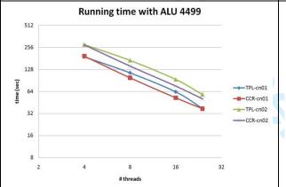
Fig. 17. Execution Time of CCR vs. TPL for Multi-Dimensional Scaling using 4499 Alu sequences on 24 core Intel vs. AMD machines
