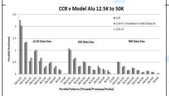
Fig. 8. Parallel Overhead f as a function of pattern tXmXn for three samples of respectively 12,500 25.000 and 50,000 AluY sequences in the case m=1 of threading internal to node. We show for each pattern, the CCR measurement followed by the two factor and single factor model.
