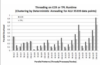
Fig. 5. Parallel Overhead for 35399 AluY sequence clustering for cases of pure threading in the node
