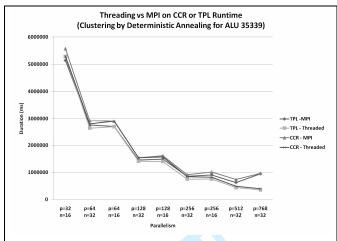
Fig. 4. Execution Time of Clustering Code for selected parallelism *p* and node counts *n*. Shown are CCR and TPL internal threading as well as intranode MPI implemented in these two frameworks
