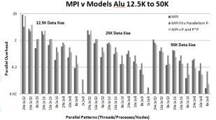
Fig. 11. Parallel Overhead f as a function of pattern tXmXn for three samples of respectively 12,500 25.000 and 50,000 AluY sequences in the case t=1 of MPI internal to node. We show for each pattern, the CCR measurement followed by the single factor and two factor model.
