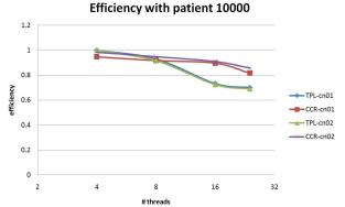
Fig. 20. Parallel Efficiency comparing CCR and TPL for Multi-Dimensional Scaling using 10,000 pt patient data on 24 core Intel and AMD machines
