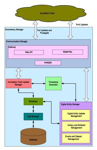
Figure 1. Hybrid Consistency Framework Architecture
