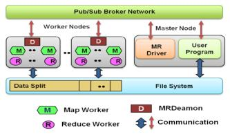
Fig. 1. Overall architecture of Twister
