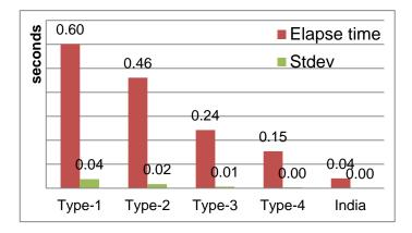
Fig. 5. Elapse time of k-means: 5 configurations - virtualized cluster systems (4 configurations) and a physical cluster system (1 configuration)
