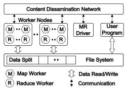
Figure 4. Components of the CGL-MapReduce
