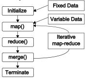
Figure 5. Computation phases of CGL-MapReduce
