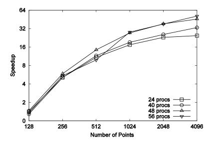
Figure 13. Speedup of MPI\_SMACOF on combine nodes
