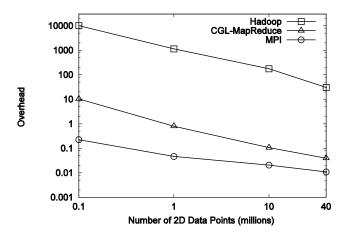
**Figure 7.** Overheads associated with Hadoop, CGL-MapReduce and MPI for Kmeans clustering – iterative MapReduce - (Both axes are in log scale)
