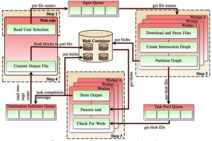
Figure 4. Crayons GIS vector overlay processing architecture.
